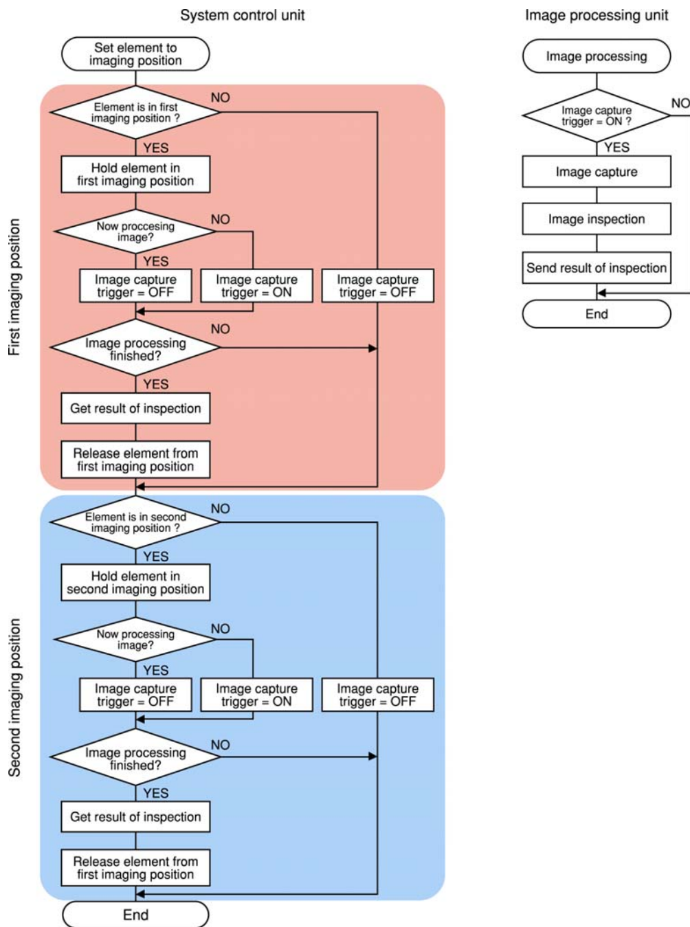
Fig. 14 Flow chart of image inspection
