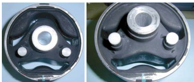
Fig. 15 Engine mount after endurance test
