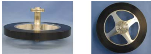
Fig. 7 Rotor for cyclic stress test
