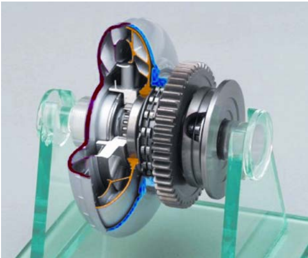
Fig. 5 Cutaway model of torque converter
