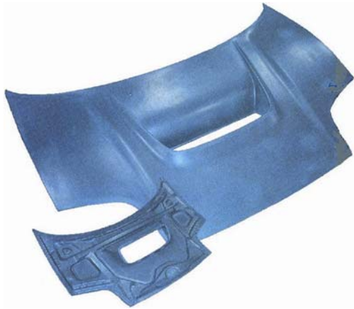
Fig. 12 External view of CFRP hood
