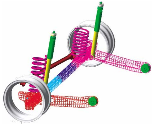
Fig. 11 Suspension model with multi FEM segments
