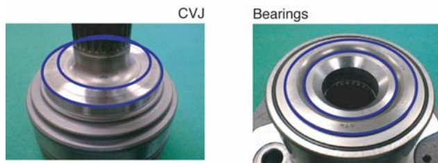
Fig. 24 Damage of contact face with \text{MoS}_2 grease
