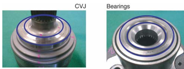
Fig. 25 Damage of contact face with rust-proof lubricant
