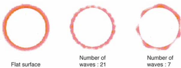
Fig. 4 Surface condition of CVJ
