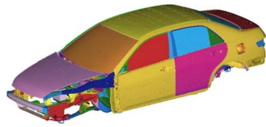
Fig. 14 FE model of trimmed body
