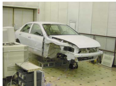
Fig. 11 Experimental trimmed body
