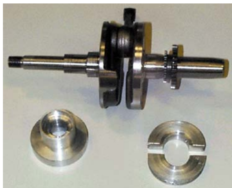
Fig. 21 Crankshaft with hydro bearing
