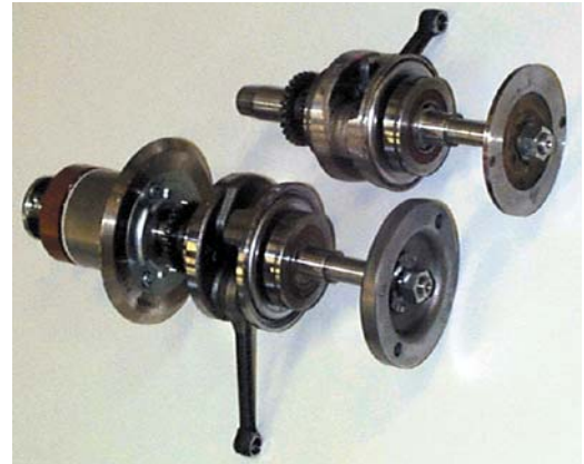
Fig. 17 Comparison between original and modified crankshaft
