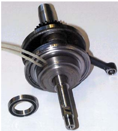
Fig. 20 Crankshaft with water-cooled bearing
