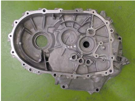
Fig. 6 Appearance of prototype of magnesium clutch case using AE62-Ca
