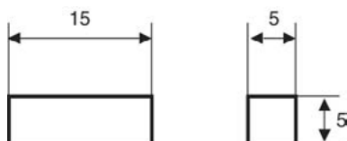
Fig. 5 Heat expansion test specimen
