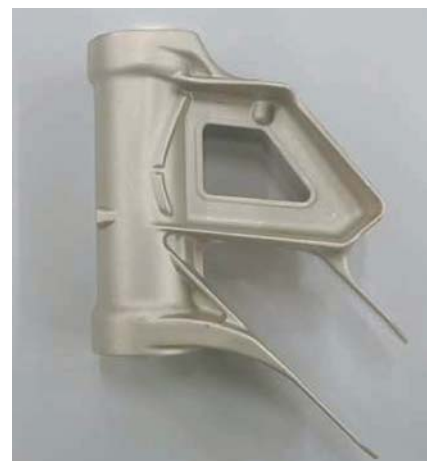
Fig. 24 Forging aluminum steering head pipe
