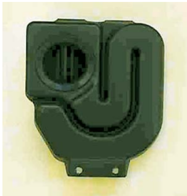
Fig. 21 Upper view of water chamber (Resonator)
