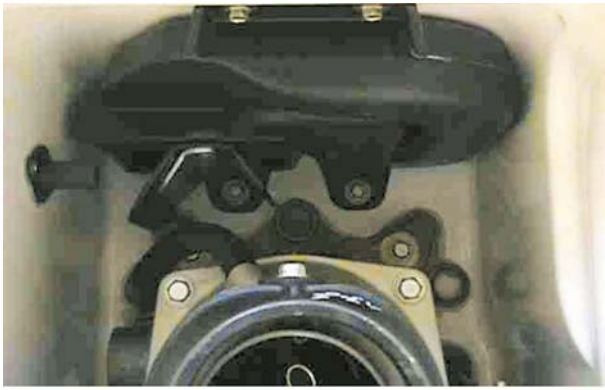
Fig. 20 Installed appearance of water chamber (Resonator)
