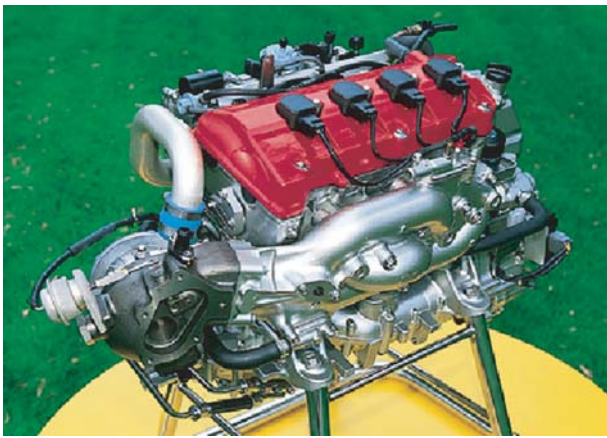
Fig. 3 F-12X Engine appearance
