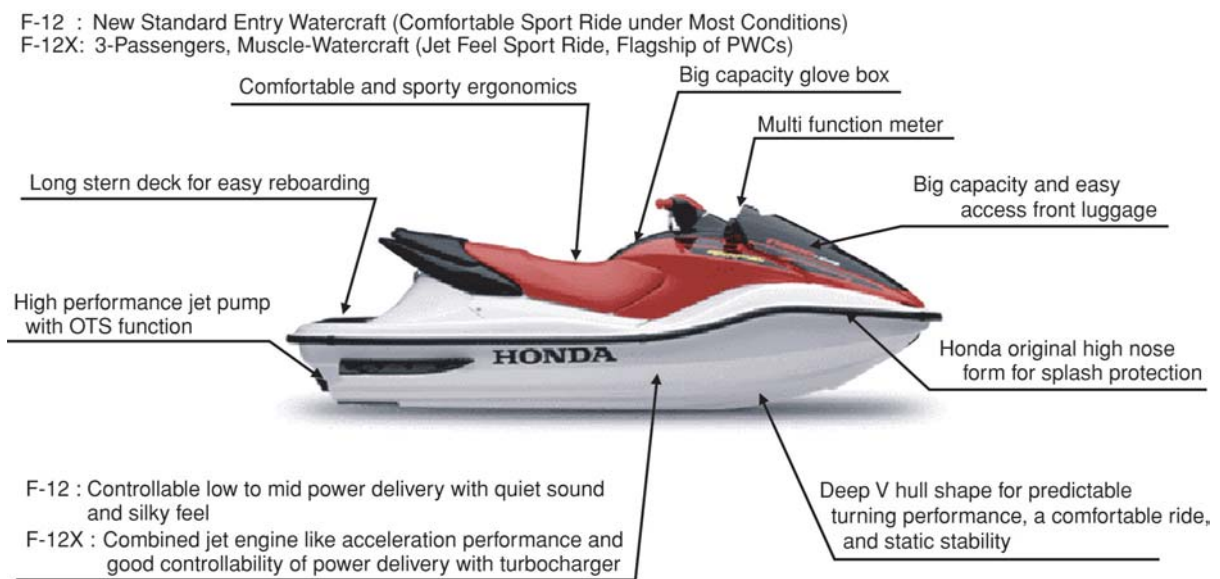
Fig. 2 Development concepts and features for AquaTrax
