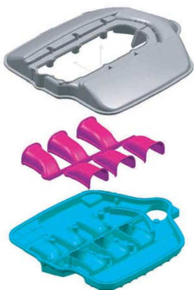
Fig. 12 Structure of inlet manifold
