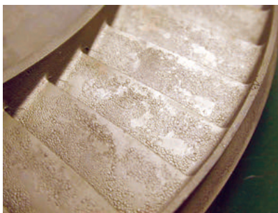
Fig. 10 Orange peel (casting)
