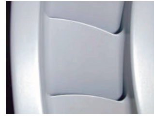
Fig. 22 Finished surface of SLA model (Primer coated)
