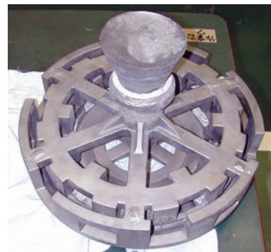
Fig. 8 As-cast turbine nozzle with gating system
