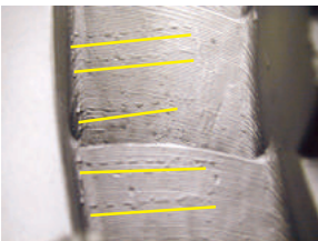
Fig. 18 Layer mark and remains of support (casting)
