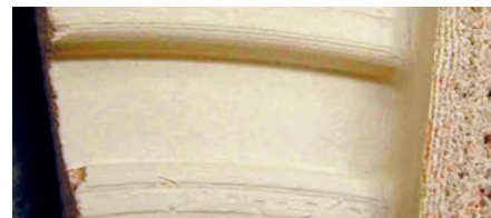
Fig. 14 No adhesion (Air blowing and air vent)
