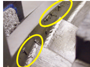
Fig. 19 Remnants of removed support (casting)
