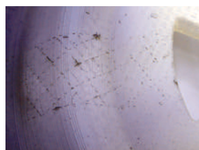
Fig. 21 Primer coated surface of SLA model (Remains of support)
