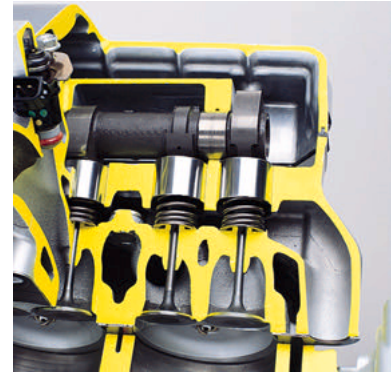
Fig. 9 Parallel two-valve train system
