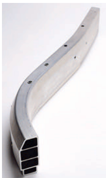
Fig. 19 Spar section of frame
