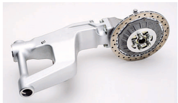
Fig. 23 Single-supported swing-arm (Pro-arm)
