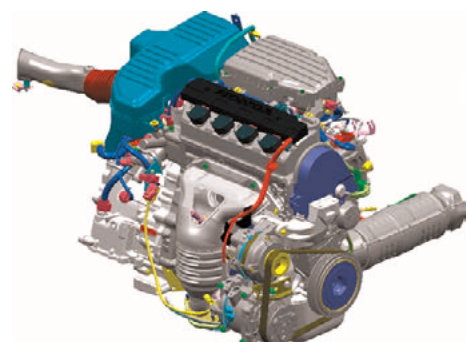
Fig. 3 View of 2001 model year lean-burn engine
