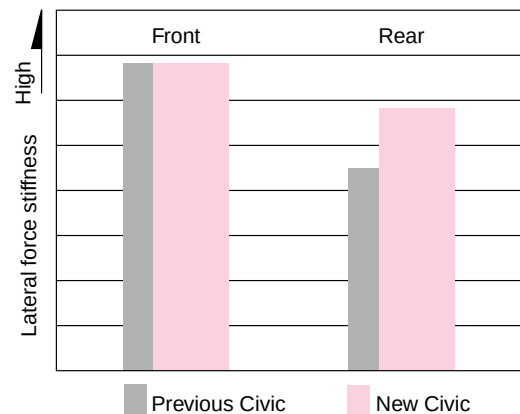
Fig. 11 Suspension lateral stiffness at tire contact point
