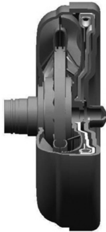
Fig. 11 Side view of developed torque converter
