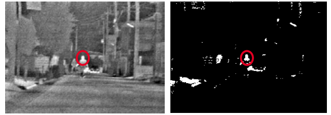
Fig. 8 Infrared image and result of two-level rendition under summer time conditions
