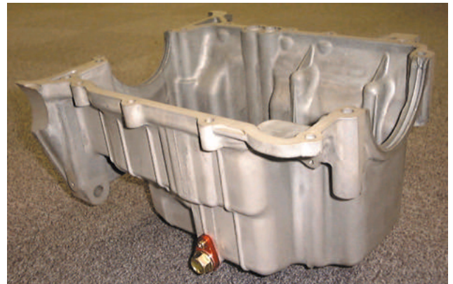
Fig.15 Appearance of magnesium oil pan using ACM522 alloy
