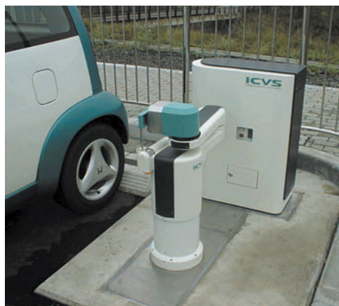
Fig.1 Inductive charger and automatic connecting unit
