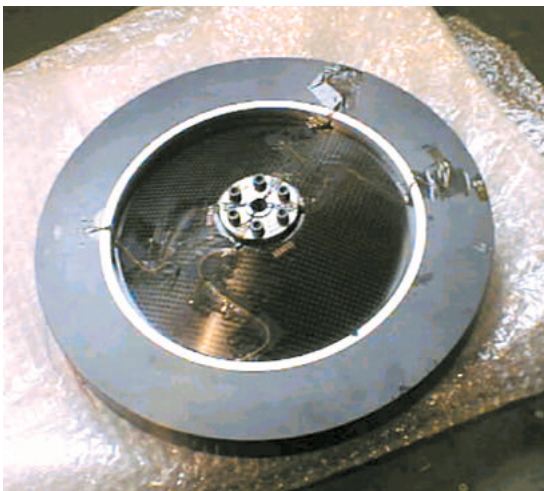
Fig.14 Rotor with strain gauge
