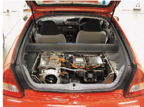
Fig.7 Rear layout of IMA system
