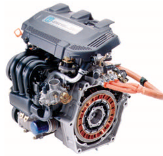
Fig.6 IMA power unit
