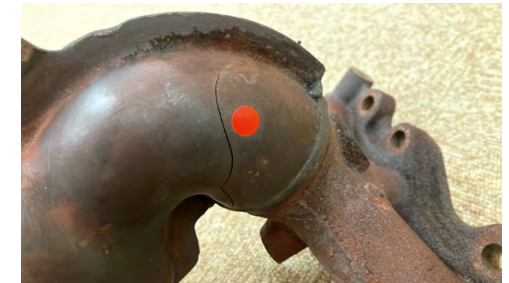
Cracked exhaust manifold of Honda Life mini-vehicle made in 1999
