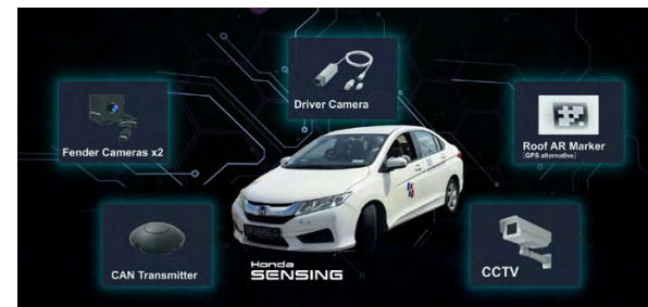
IDC system configuration
