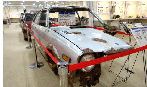
Rust on the body of a Honda Civic made in 1981
