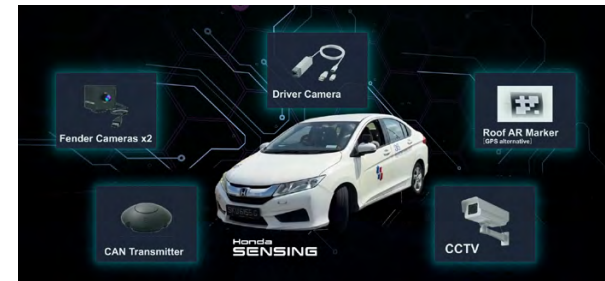
IDC system configuration
