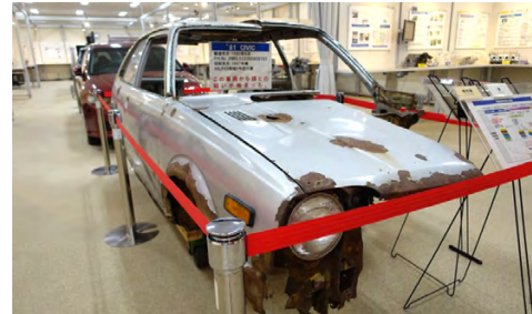
Rust on the body of a Honda Civic made in 1981
