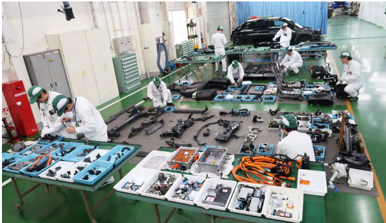
Verification of parts following durability testing
