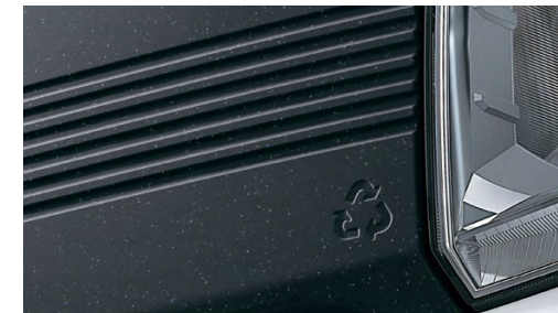
Front grille parts made of "recycled bumper material"
