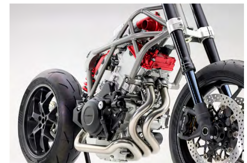
V3 engine with electrical compressor
