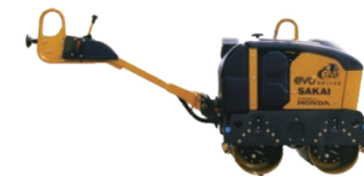
"eGX" and "Honda Mobile Power Pack e:" equipped SAKAI HEAVY INDUSTRIES, LTD. Electric Walk- Behind Roller "HV620 evo"
