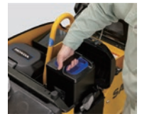
"eGX" and "Honda Mobile Power Pack e:" equipped SAKAI HEAVY INDUSTRIES, LTD. Electric Walk- Behind Roller "HV620 evo"
