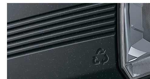
Front grille parts made of “recycled bumper material”
