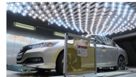
Bench environment test Analyses are conducted in road environments found around the world, from low temperatures to under the scorching sun, to humid conditions, traffic jams and high speeds.
