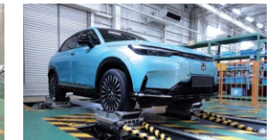
Bench vibration test Actual vehicle vibrations are reproduced on a testing bench together with analyzing issues.
