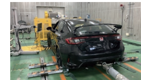
Exhaust gas and mode driving verification The compliance of exhaust gas components with emissions regulations and proper system operation during mode driving are verified.
