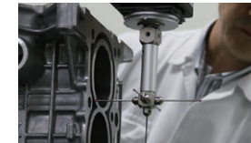
Measuring part precision Parts' dimensional precision is verified using 3D measurement and the latest roundness measurement equipment.
