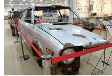
Rust on the body of a Honda Civic made in 1981
