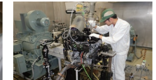
Testing engine functionality and performance The functionality and performance of assembled engines are verified on a bench.
