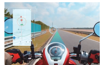
Demonstration test of a motorcycle hazard notification technology using infrastructure cameras (at Honda's test course)
