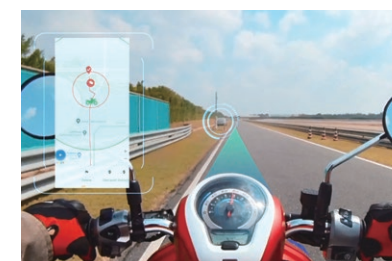
Demonstration test of a motorcycle hazard notification technology using infrastructure cameras (at Honda's test course)
