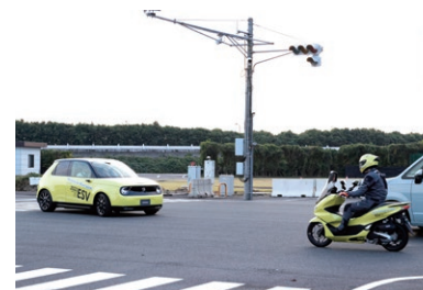
Demonstration of an accident scenario involving a right-turning vehicle and a motorcycle proceeding straight ahead at an intersection (at Honda's test course)
