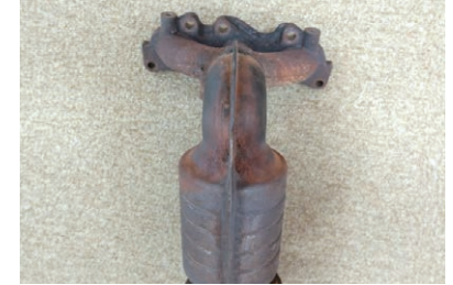
Cracked exhaust manifold of Honda Life mini vehicle made in 1999
