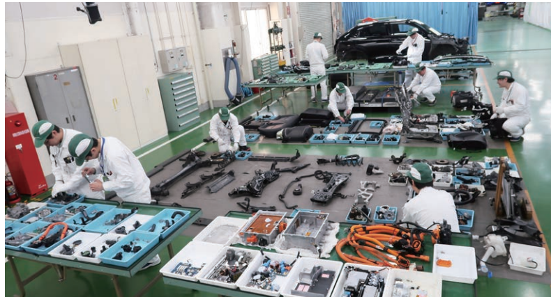
Verification of parts following durability testing
