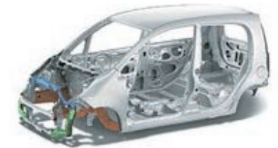
Advanced Compatibility Engineering (ACE) body structure
