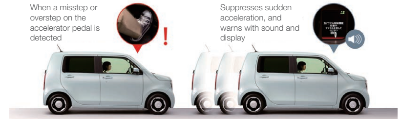
Sudden Acceleration Suppression Function (N-WGN, Japan)
