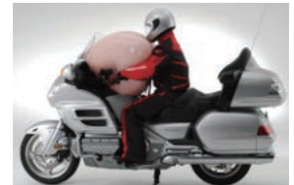
Mass-produced airbag system for motorcycles
