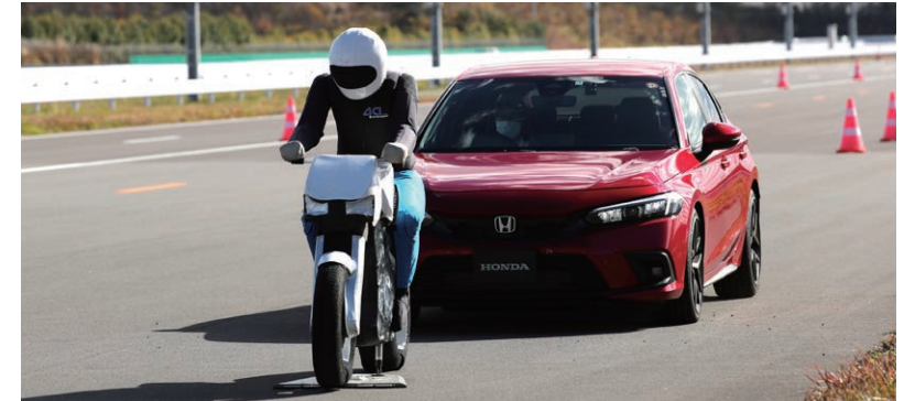
Honda SENSING with motorcycle detection function
