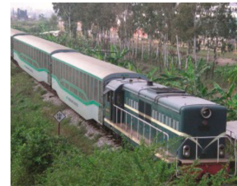
Special freight cars for transporting automobiles
