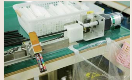
Karakuri -style innovation at work: A device that uses a store-bought pen to ensure that parts are marked properly for subsequent processing
