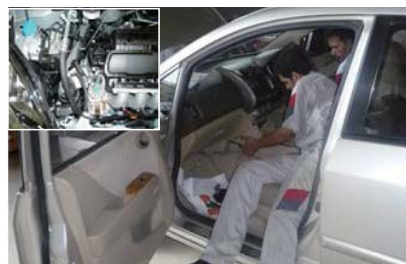
Technicians use the mount canceller to diagnose vehicle issues. Vibrations are transmitted to the car's interior, allowing the problem to be accurately diagnosed.
