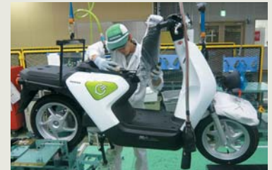
The EV-neo is manufactured at Honda's Kumamoto Factory, its leader motorcycle plant. Its motor is manufactured on the same production line as the Monpal electric cart.
