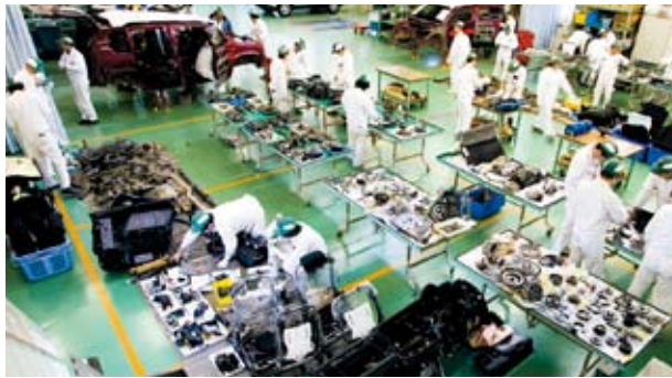
Full disassembly inspection
