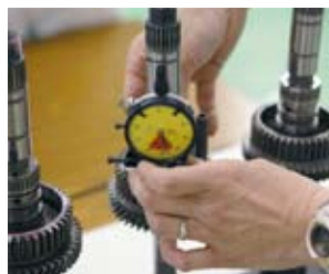
Introduced to assure outstanding quality, these jigs enable easy measurement of inside and outside diameters.
