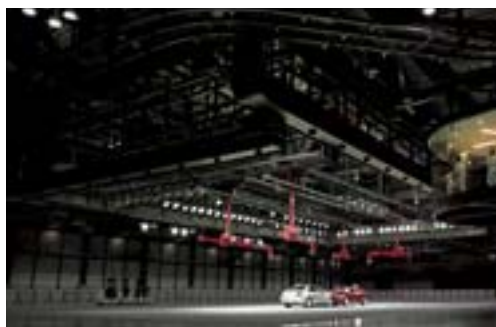
The indoor omnidirectional Real World Crash Test Facility
