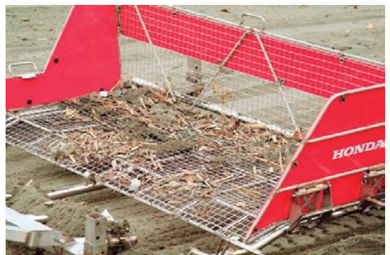
A simple yet ingenious towable sand screen separates litter from sand
