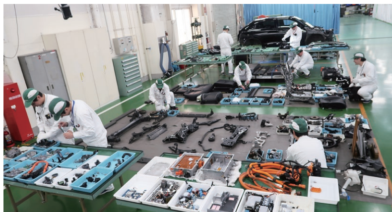
Verification of parts following durability testing
