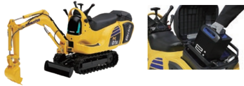
Komatsu Ltd.'s PC01E-1 Electric Micro Excavator Equipped with Honda Mobile Power Pack e:
