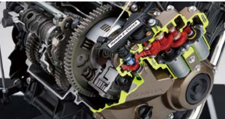
Electronically Controlled Clutch Technology for Motorcycles: E-Clutch
