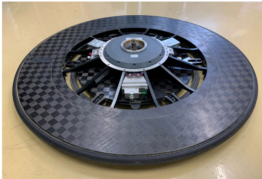
Push power measurement system for racing wheelchairs
